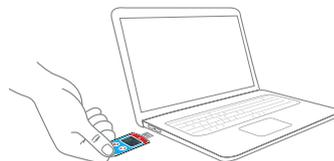
**03** Connect stopped logger directly to USB port
